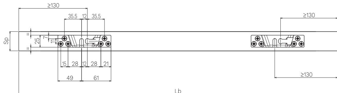
**Hp** = door leaf height (mm) - **Lp** = door leaf width (mm) - **Lb** = track length (mm) - **Sp** = door leaf thickness (mm)
